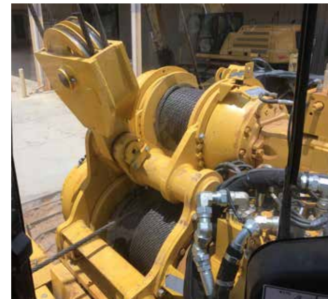
Good view to winch drums for spooling
