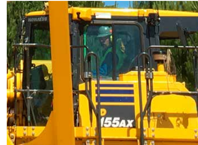
Comfortable air-conditioned and heated ROPS cab has large glass area for good visibility
