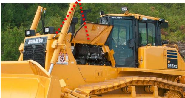
2) With the key switch ON, Press F6, scroll to the MACHINE SETTING menu and select FAN REVERSE MODE by pressing F6 again
