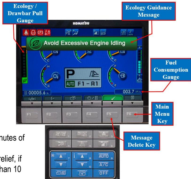
On-screen, Ecology guidance messages disappear after five seconds or when the F5 key is pushed. Ecology Guidance is easily turned off in the “Energy Saving Guidance” user settings tab if operators prefer not to have messages displayed on screen.
