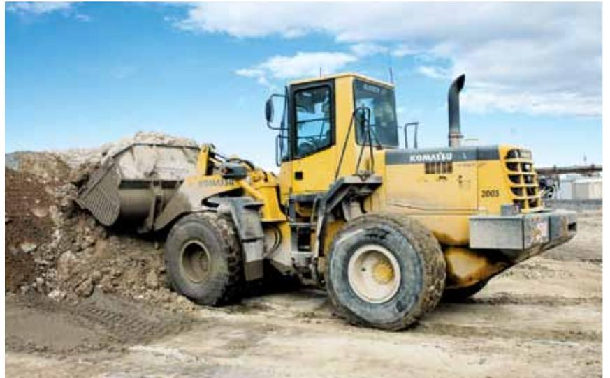
Companies such as Brannan Sand and Gravel use older Komatsu wheel loaders to charge crushers and as general-purpose machines. “What I’m looking for is reliability and fuel efficiency — machines I can count on every day and that won’t break me paying for diesel fuel — and that’s what I get from our Komatsu machines,” said Aggregate Production Supervisor Jim Thompson.
